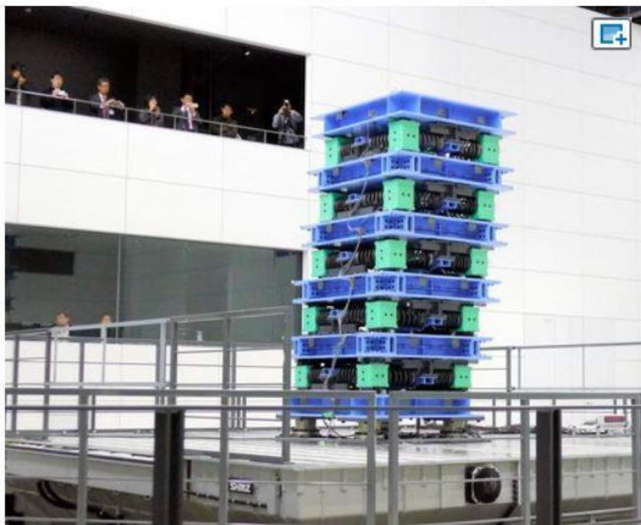
A 1/40 scale model of a building undergoes a seismic test at a Shimizu Corp. facility in Tokyo on March 4. (Takashi Kamiguri)
